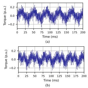
**Fig. 7.** Torque waveforms (related to the rated torque) for *motor* 2 under AM for the voltage change  $\delta u = 94\%$ , the modulation frequency  $f_m = 26$  Hz, and the symmetrical (a) and asymmetrical (b) rectangular modulation.
