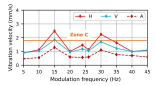
**Fig. 14.** Measured broadband vibration velocity for the voltage change  $\delta_u = 0.94\%$  in the horizontal (H), vertical (V), and axial (A) directions versus the frequency of the asymmetrical rectangular voltage modulation.
