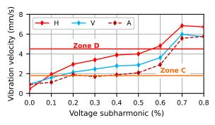
**Fig. 12.** Measured broadband vibration velocity in the horizontal (H), vertical (V), and axial (A) directions versus the value of the voltage subharmonic for the frequency  $f_{sh} = 20$  Hz.
