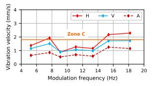
**Fig. 16.** Measured broadband vibration velocity in the horizontal (H), vertical (V), and axial (A) directions versus the modulation frequency, for the modulating function with ramp changes and  $P_{st} = 1$ .
