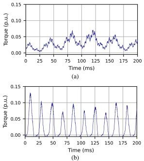
**Fig. 6.** Torque waveforms (related to the rated torque) for *motor 1* under *AM* for the voltage change  $\delta u = 0.94\%$ , the modulation frequency  $f_m = 26$  Hz, and the symmetrical (a) and asymmetrical (b) rectangular modulation.
