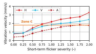
**Fig. 17.** Measured broadband vibration velocity in the horizontal (H), vertical (V), and axial (A) directions versus the short-term flicker severity  $P_{st}$ , for the modulating function with ramp changes and  $f_m = 15.385$  Hz (T = 65 ms).
