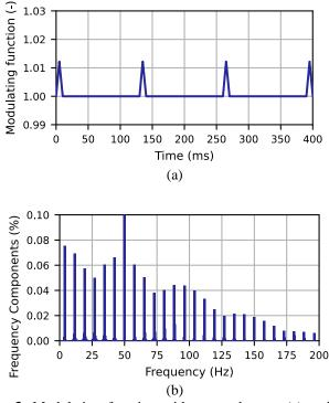
**Fig. 3.** Modulating function with ramp changes (a) and the corresponding voltage spectrum (b) for the modulation period  $T = 130 \text{ ms} (f_m = 7.692 \text{ Hz}).$
