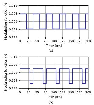
**Fig. 1.** Sample modulating functions for  $f_m = 26$  Hz and a duty cycle equal to 50% (a) or 25% (b).
