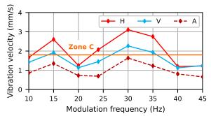
**Fig. 15.** Measured broadband vibration velocity for the voltage change  $\delta_u = 1.33\%$  in the horizontal (H), vertical (V), and axial (A) directions versus the frequency of the asymmetrical rectangular voltage modulation.
