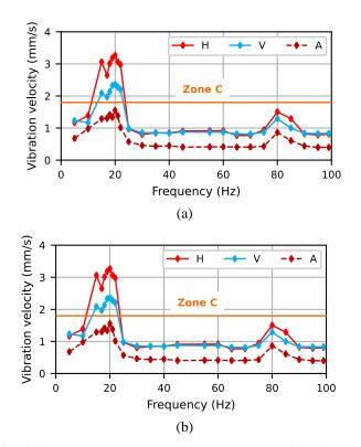
**Fig. 10.** Measured broadband vibration velocity in the horizontal (H), vertical (V), and axial (A) directions versus the frequency of voltage subharmonics and interharmonics  $f_{sh/ih}$ , for *SaIs* values of  $u_{sh}/i_{sh} = 0.3\%$  (a) and  $u_{sh}/i_{sh} = 0.1\%$  (b).
