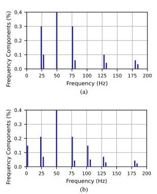
**Fig. 2.** Spectra of the voltage waveforms for the symmetrical modulating function presented in Fig. 1a (a) and asymmetrical modulating function shown in Fig. 1b (b).
