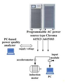
Fig. 5. Simplified diagram of the measurement stand.
