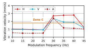
**Fig. 13.** Measured broadband vibration velocity for the voltage change  $\delta_u = 0.94\%$  in the horizontal (H), vertical (V), and axial (A) directions versus the frequency of the symmetrical rectangular voltage modulation.
