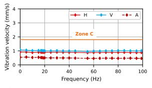
**Fig. 11.** Measured broadband vibration velocity in the horizontal (H), vertical (V), and axial (A) directions versus the frequency of voltage subharmonics and interharmonics  $f_{sh/ih}$ , for *SaIs* value of  $u_{sh}/i_{sh} = 0.3\%$  and full load.
