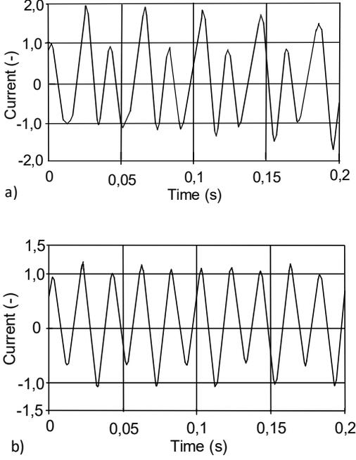
Fig. 9. Waveforms of the supply current for *Case A* (a) and *Case B* (b) and voltage containing subharmonic of frequency  $f_{sh} = 26$  Hz and  $U_{sh} = 1\% U_{rat}$ . The current value is related to the amplitude of the fundamental harmonic.
