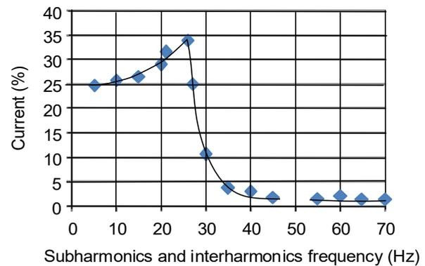
Fig. 13. Subharmonic and interharmonic content in the supply current vs. frequency of voltage subharmonics and interharmonics for Case A and  $U_{sh}, U_{ih}=1\% U_{rat}$ . The frequency components are related to the rated current.
