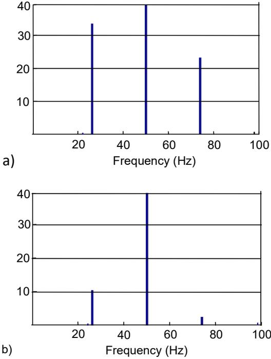
Fig. 10. Spectra of the supply current for *Case A* (a) and *Case B* (b) and voltage containing subharmonic of frequency  $f_{sh} = 26$  Hz and  $U_{sh} = 1\% U_{rat}$ . The frequency components are related to the rated current.
