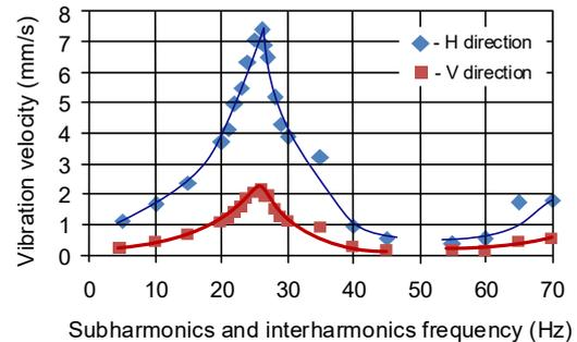
Fig. 4. Broad-band vibration velocity vs. subharmonic and interharmonic frequency for *Case A*,  $U_{sh/ih} = 1\% U_{rat}$ , direction H and V.
