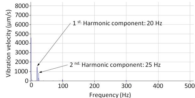
Fig. 12. Spectrum of vibration velocity for Case A, direction H frequency  $f_{ih}=70$  Hz and  $U_{sh}=1\% U_{rat}$ .
