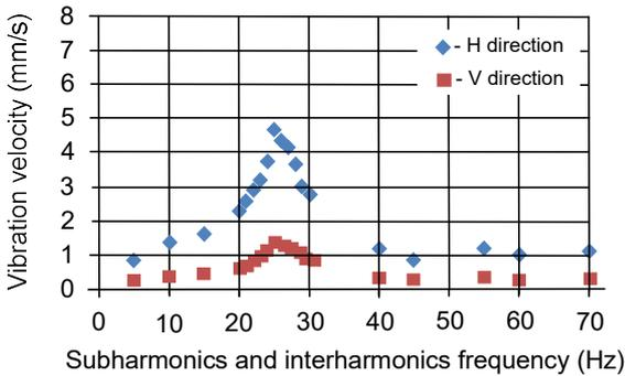
Fig. 7. Broad-band vibration velocity vs. subharmonic and interharmonic frequency for Case A,  $U_{sh/ish}=0.5\%$ , direction H and V.
