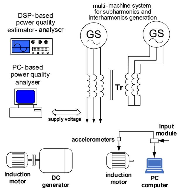
Fig. 2. A simplified diagram of the measurement stand.
