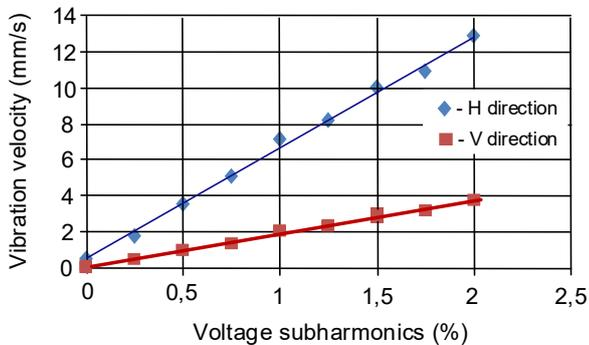
Fig. 14. Broad-band vibration velocity vs. subharmonic voltage, for Case A, direction H, V and frequency  $f_{sh}=26$  Hz.
