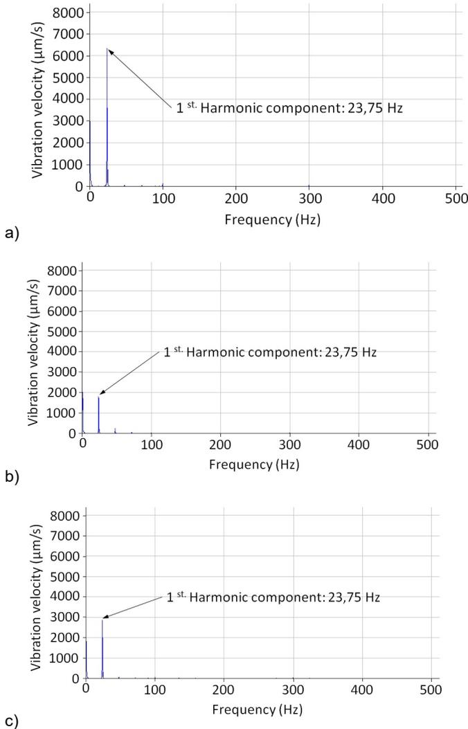
Fig. 11. Spectra of vibration velocity for Case A, direction H (a), V (b), L (c) frequency  $f_{sh}=26$  Hz and  $U_{sh}=1\% U_{rat}$ .
