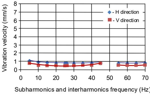
Fig. 6. Broad-band vibration velocity vs. subharmonic and interharmonic frequency for Case C,  $U_{sh/ish}=1\% U_{rats}$ , direction H and V.
