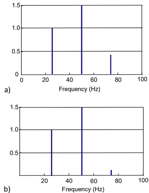
Fig. 8. Spectra of the testing voltage for Case A (a) and Case B (b) and voltage containing subharmonic of frequency  $f_{sh}=26$  Hz and  $U_{sh}=1\% U_{rats}$ . The frequency components are related to the rated voltage.
