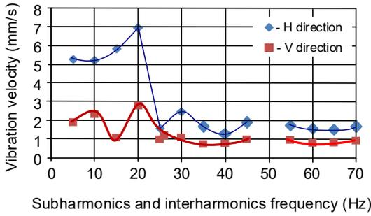
Fig. 5. Broad-band vibration velocity vs. subharmonic and interharmonic frequency for Case B,  $U_{sh/ish}=1\% U_{rats}$ , direction H and V.
