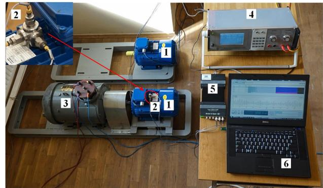
Fig. 1. Photograph of the investigated motors with measurement equipment. 1 – Induction motors, 2 – Accelerometers, 3 – DC generator, 4 – Power quality estimator analyser, 5 – Input module, 6 – PC computer with Bruel & Kjar software PULSE
