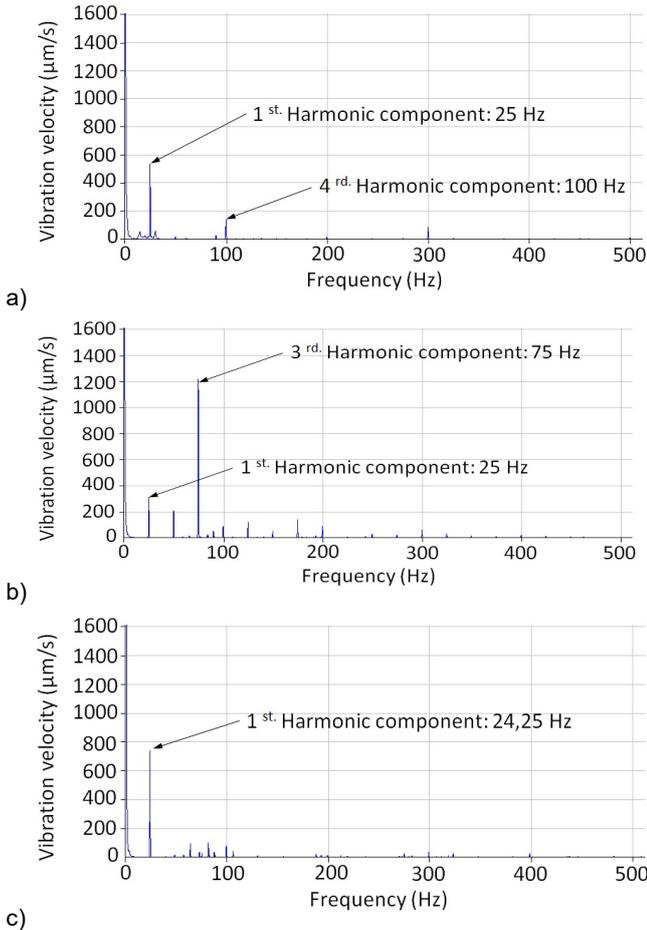
Fig. 3. Spectrum of vibration velocity under sinusoidal supply, for direction H and *Case A* (a), *Case B* (b), *Case C* (c).
